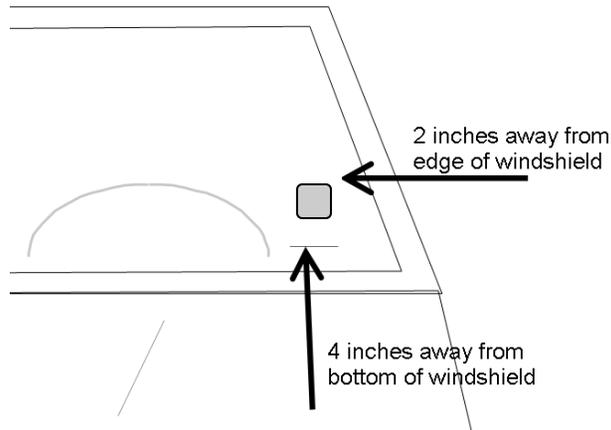
**NOTE: The AVI Tag must be installed with the blank side facing the outside of the vehicle, toward the AVI Reader.**
