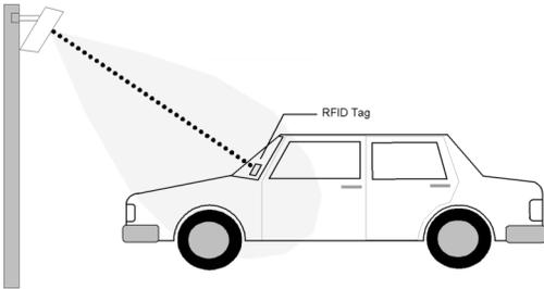
The AVI Reader is mounted on a pole, wall, or ceiling near a gated parking area entrance or exit.
